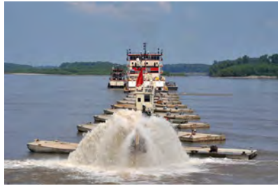
Sediment "Recharge" via Dredging
